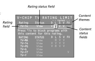
Pressing RESET on the remote will reset all ratings to View and V.
